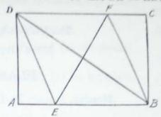
33 a One method of laying out a corner B for a rectangular field is as follows: Stakes are set at points B and F, 50 feet apart. A third stake is then set at D, 50 feet from both B and F. A fourth stake is set at E, in line with F and D and 50 feet from D. Explain why the line through B and E is perpendicular to the line through B and F. [3]
