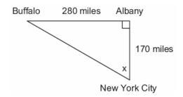
*a* If an engineer wants to design a highway to connect New York City directly to Buffalo, at what angle, *x*, would she need to build the highway? Find the angle to the *nearest degree*.
